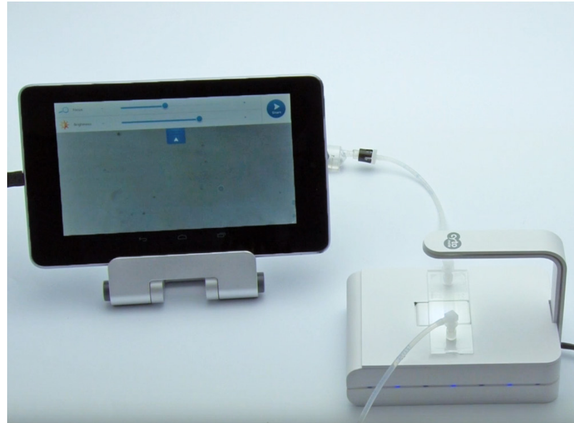
Figure 5. The open design of the CytoSMART™ Lux2 Duo Kit enables easy monitoring of cells cultured inside microfluidic devices. In this case, the flow and attachment of cells within a microfluidic chip is monitored.
