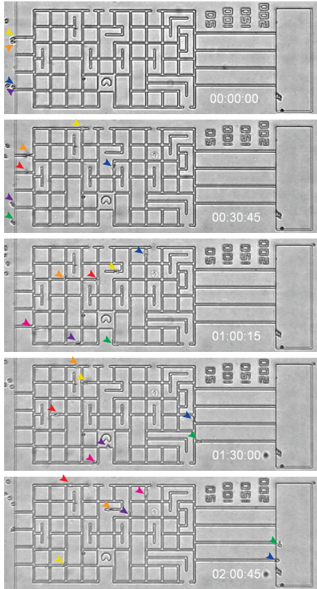
Figure 4. Human neutrophils navigate their way through a microscopic size maze (total maze size is 0.8 mm) towards a reservoir with chemoattractant on the right. Colored arrowheads indicate the same neutrophils at different timepoints. The speed and directionality of neutrophil movement towards the chemoattractant is followed using the CytoSMART™ Lux2 Duo Kit.
