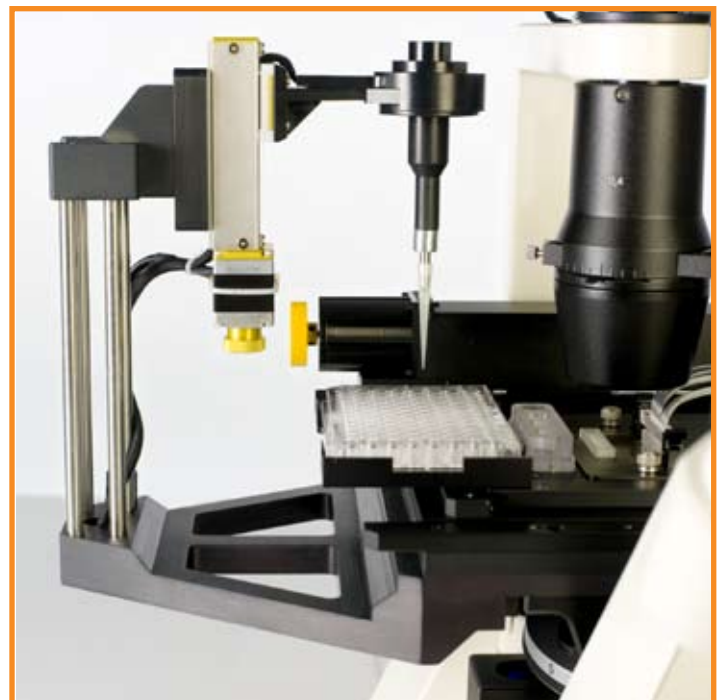
VenaFlux™ Robotic Arm integrates with 96-well plates.
