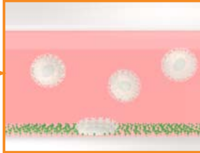
Illustration: Cell adhesion inside ligand-coated microchannel of Vena8™ Biochip
