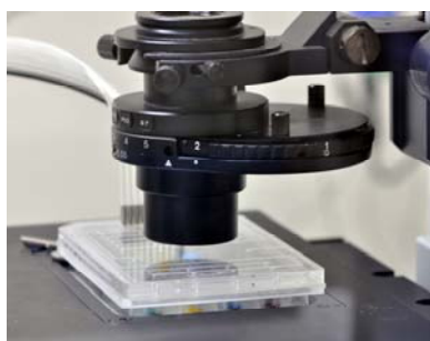
Figure 2. Plate with Manifold on Stage
